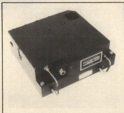
Fig. 2 Latest design Marisat uplink/downlink RF subsystem.
